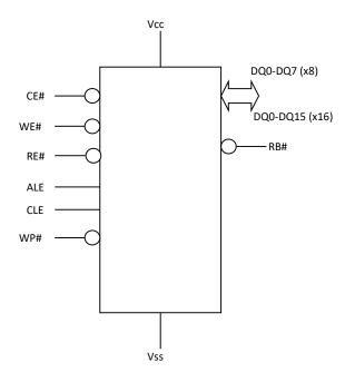
Figure 1: Logic Diagram
