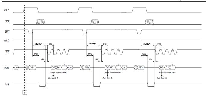
Figure 13: read cache timings, end of cache operation
