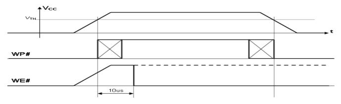
Figure 27: Power on and Data Protection timings
