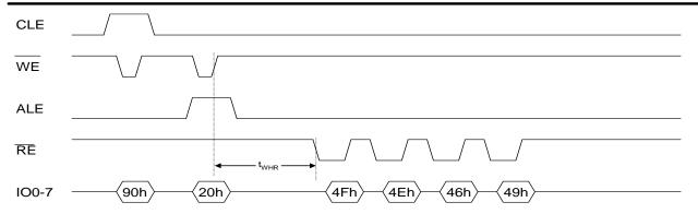
Figure 22: ONFI signature timing diagram
