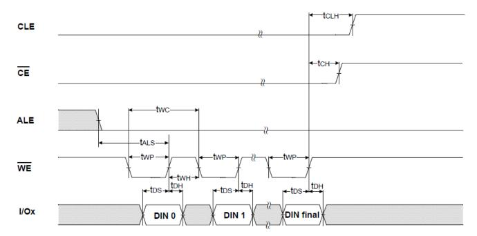
Figure 5: Input Data Latch Cycle
