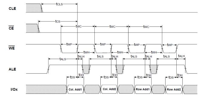
Figure 4: Address Latch Cycle
