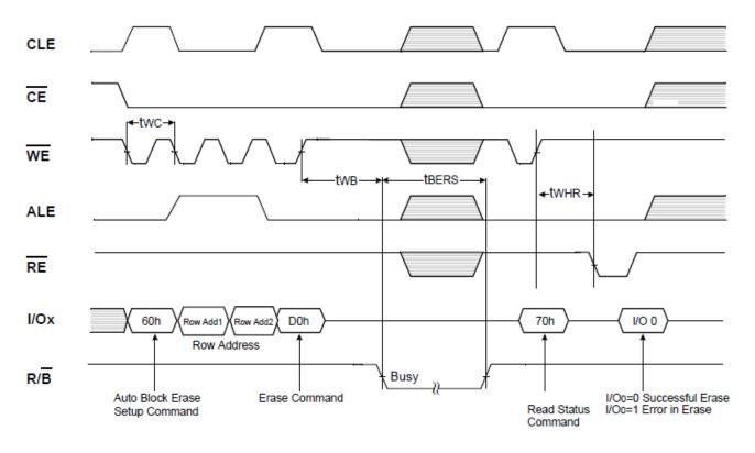
Figure 20: Block Erase Operation (Erase One Block)
