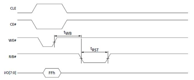
Figure 23: Reset operation timing
