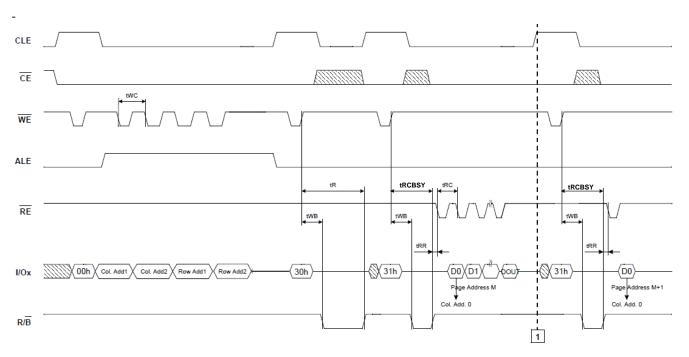
Figure 12: read cache timings, start of cache operation
