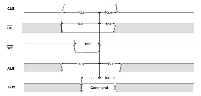
Figure 3: Command Latch Cycle
