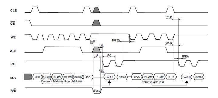
Figure 16: Copy Back read with optional data readout
