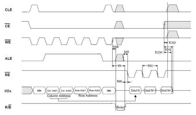
Figure 10: Read Operation intercepted by CE#
